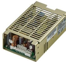
U Type (With Top cover): 3.2(W) x 5(L) x 1.66(H) inches.
